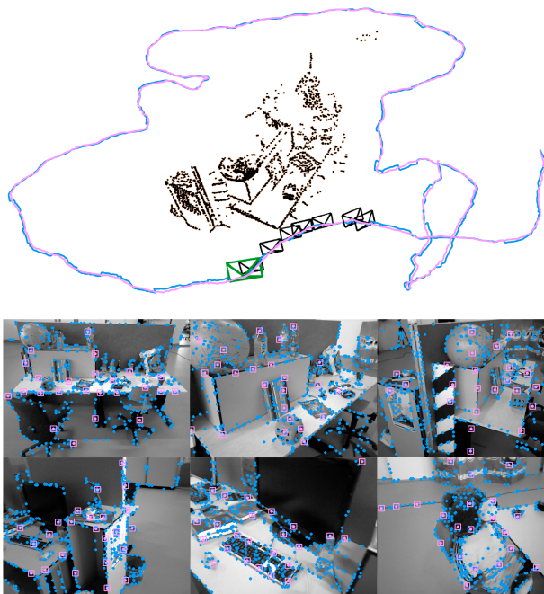
Figure 1: Top: Trajectories and maps estimated by our RGB-D odometry (ID-RGBDO) in two cases: tracking 500 image points (blue), and tracking only the 24 most informative points (magenta) with considerable computational savings. The difference between the two is almost unnoticeable. Bottom: Sample frames and tracks for the 500 points case (blue dots) and the 24 most informative ones (magenta squares).
