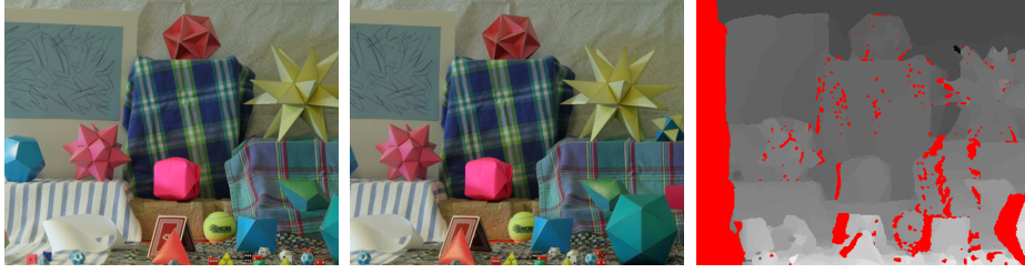
Fig. 6. The proposed method can be employed to simultaneously optimize for a displacement and an occlusion map. This problem is also too large to be solved by alternative relaxation methods on current GPUs. From left to right: (a) Left input image I_L . (b) Right input image I_R . (c) Computed disparity and occlusion map, red areas denote occluded pixels.
