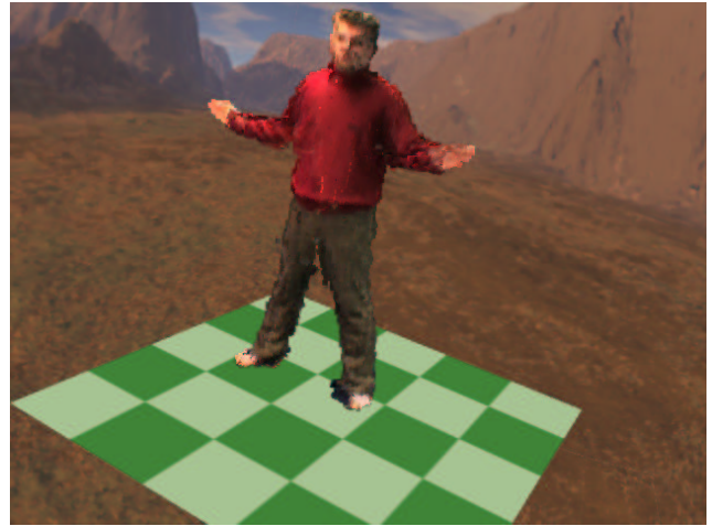
Fig. 5. Rendered view. The novel viewpoint lies directly in between two of the source cameras in Fig. 4.
