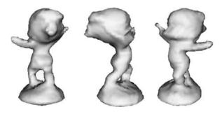
**Fig. 4** Final shape estimated using the algorithm (Jin et al. 2004a) with a combination of one positive light and one negative light. The algorithm reconstructs the 3D object more accurately (compared with Fig. 3), nevertheless the lighting configuration if not physically plausible.
