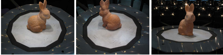
Fig. 2. Some of the input images used for 3D reconstruction. The image sequence is pretty challenging because of the presence of reflections and illumination artefacts.
