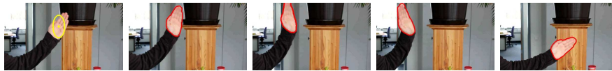
Fig. 12 Moment constraints for object tracking. The user initializes the tracking by clicking an ellipse in the first frame, the moments of which constrain the segmentation in subsequent images. A small deviation of the centroid is allowed to track the moving object. Note that this approach is generic, as no shapes have to be previously learned.
