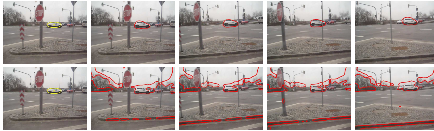
Fig. 13 Moment constraints for object tracking. The user initializes the tracking in form of an ellipse in the first frame (left), from which histograms and constraint parameters are derived. The first row shows results with moment constraints, where a deviation of the centroid is allowed from each frame to the next one to account for the object’s motion. The second row shows results of histogram based tracking without constraints. This comparison shows that moment constraints can realize acceptable real-world object tracking with no previous learning of shapes.
