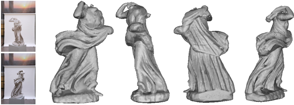
Fig. 4.12: Reconstruction from a hand-held camera. 2 out of 28 input images of resolution 2048 \times 3072 and multiple views of the reconstructed surface. Despite severe illumination variations in the input images, the creases of the cloth are recovered in high detail.
