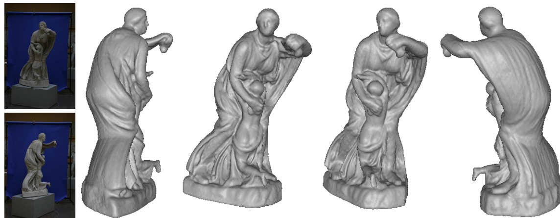
Fig. 3.14: Statue #3. 2 out of 38 input images of resolution 2048 \times 3072 and multiple views of the reconstructed 3D surface.
