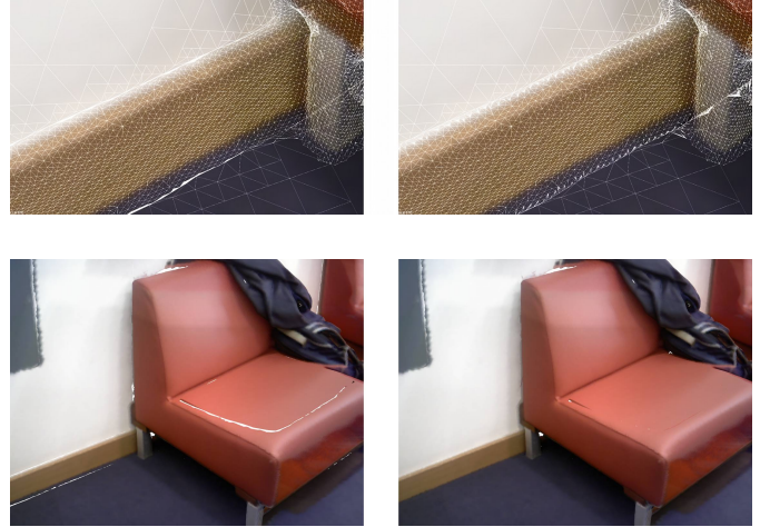
Figure 14: Joining of GPT mesh with planar segment triangulations. Left shows unjoined segments and right shows segments joined with interpolated boundary vertices.
