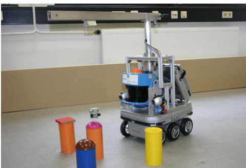
Fig. 1. Demonstrator scenario of the EU project MACS [4]. A goal of MACS is to explore affordance-inspired perception and learning for mobile robots related to J.J. Gibson's theory. The shown robotic agent KURT3D should perceive, learn and utilize its environment in a functional way.
