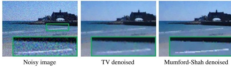
Fig. 2 While total variation regularization (center) induces a contrast loss, truncated regularizers like the Mumford-Shah model (right) better preserve discontinuities and contrast. The right image was computed using a convex relaxation of the vectorial Mumford-Shah model proposed in [64].
