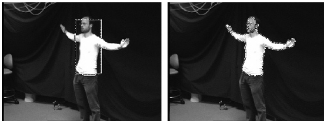
Figure 2: Silhouette extraction based on level set functions. Left: Initial segmentation. Right: Segmentation result.
