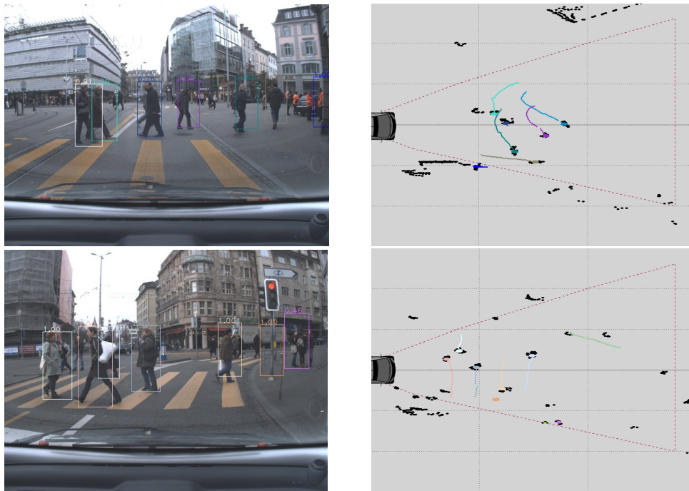
Fig. 7. Qualitative results from dataset 1 and 2 showing pedestrian crossings. The colored boxes in the image describe different tracks and probability levels; the size of the filled circle in the tracking figure is proportional to pedestrian detection confidence. It is important to notice that highly occluded pedestrians are also successfully detected and tracked.
