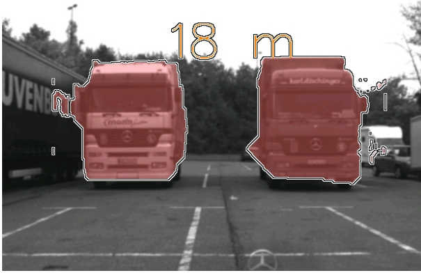
Fig. 10. Graph Cut Segmentation. The obstacles in 18 m distance are accurately separated from the background by means of segmentation carried out on relative image motion.
