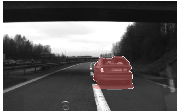
Fig. 11. Segmentation of moving vehicle. As the car turns into the field of view of the radar sensor, it is verified and segmented by computer vision. Recall that segmentation is purely based on monocular vision analyzing relative image motion. This examples demonstrates the benefit of sensor collaboration in complex situations.
